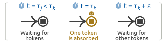
Figure 23. Token absorption in an end event.
